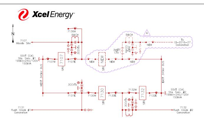
Figure 3: GI-2016-27 Physical Interconnection at Pronghorn Switching Station
